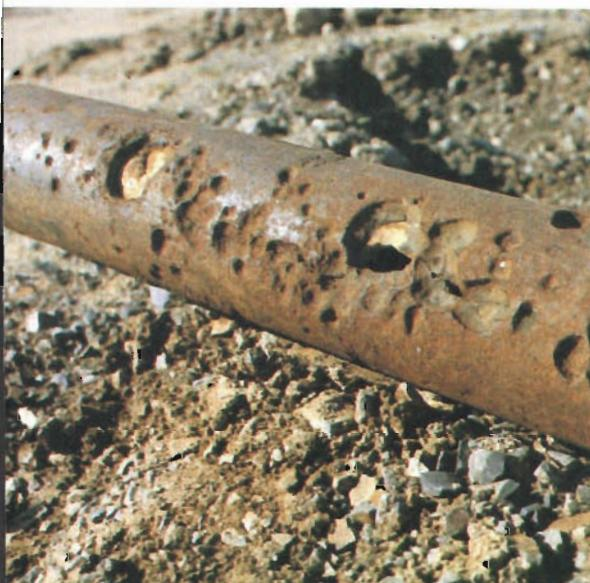
Damage to water pipe by electrolysis.
