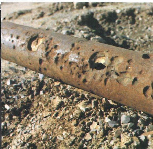
Damage to water pipe by electrolysis.
